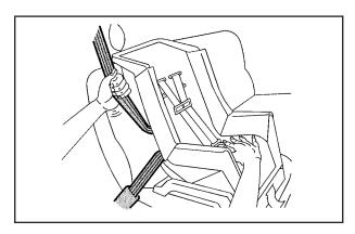
To tighten the belt, push down on the child restraint, pull the shoulder portion of the belt to tighten the lap portion of the belt and feed the shoulder belt back into the retractor. If you are using a forward-facing child restraint, you may find it helpful to use your knee to push down on the child restraint as you tighten the belt. You should not be able to pull more of the belt from the retractor once the lock has been set.
